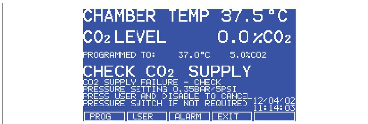
Fig. 5-9: *CHAMBER ALARM* to check CO<sub>2</sub> supply
